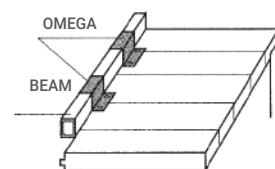
On the transversal joints, the panels will be supported or hung according to the characteristics of the place where the cold room is installed.
