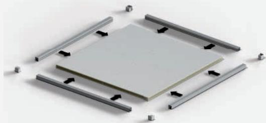
If the cold room has no floor, the ground of the cold room perimeter must be completely levelled width (E+150 mm). Fig A.
