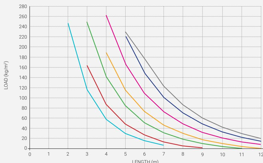
Admissible loads for these panels according to thickness, deflection  $L/200$  and standard NBE 95.
