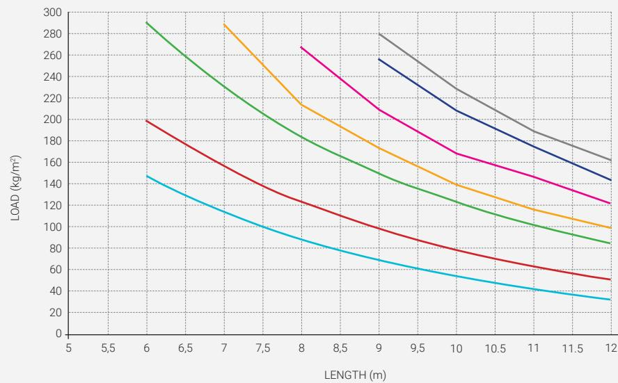
Admissible load per panel with two supports and deflection of  $l/200$ , being  $l$  the distance between supports.
